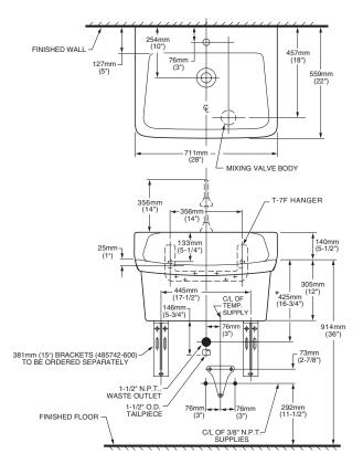
NOTES: \* DIMENSION SHOWN FOR LOCATION OF "P" TRAP IS SUGGESTED. 15" PAINTED SUPPORT BRACKETS 485742-600 AVAILABLE AND MUST BE ORDERED SEPARATELY. PROVIDE SUITABLE REINFORCEMENT FOR ALL WALL SUPPORTS.
