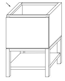
**STEP 3:** Apply adhesive on wood bracket and mounting surfaces of the cabinet
