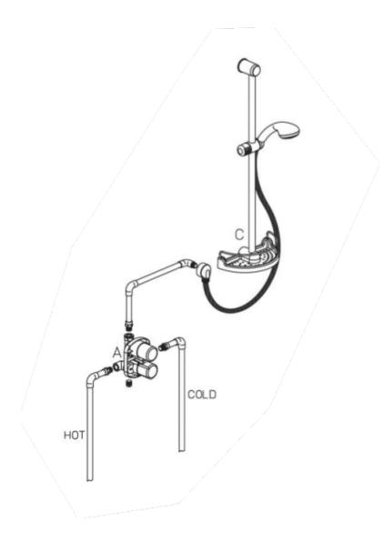
Water Harmony thermostatic valve with ¾" ceramic disk volume control Slide bar kit Rough included.
