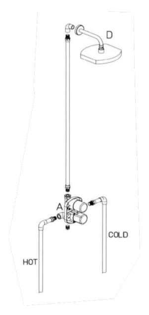
Novello thermostatic valve with 3/4" ceramic disk volume control 8" rain shower head with 12" arm Rough included.
