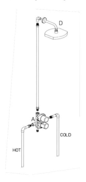
Lady thermostatic valve with 3/4" ceramic disk volume control
