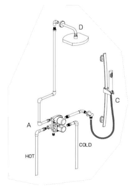
Elba thermostatic valve with 2-way diverter volume control 8" rain shower head with 12" arm Slide bar kit. Rough included.
