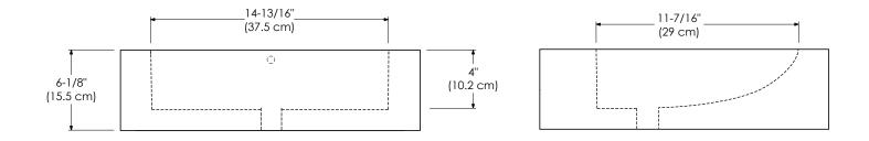
By IAPMO, ceramic lavatory warpage is defective only if warpage of flat slab out of horizontal plane exceeds 6.3 mm/m (0.25 in/ft) on all sizes OR warpage on back of lavatories that are attached to the wall exceeds 3 mm (0.13 in).
