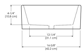
By IAPMO, ceramic lavatory warpage is defective only if warpage of flat slab out of horizontal plane exceeds 6.3 mm/m (0.25 in/ft) on all sizes OR warpage on back of lavatories that are attached to the wall exceeds 3 mm (0.13 in).
