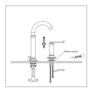
Slip the valve body's flexible hoses from the top of the sink or counter through the appropriate hole next to the spout.
