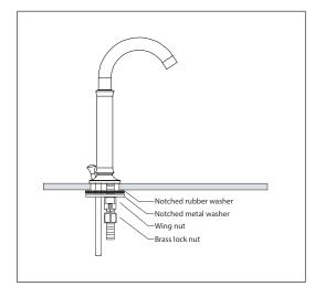
C Align spout and secure to the sink or counter surface by tightening the 2 screws on the wing nut with a Phillips head screwdriver.
