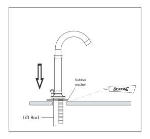
B Slip the spout mounting hardware back onto the spout. First the notched rubber washer, then the notched metal washer, (making sure the notch faces towards the back) wing nut, and brass lock nut. Insert lift rod and make sure it operates smoothly.
