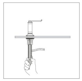
D Loop and connect the flexible hoses to the tee.
