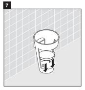
Slide the unit down onto the mounting bracket.
