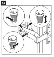
The top screw will adjust up and down.
