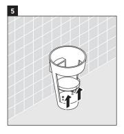
Lift the unit up and onto the mounting brackets.
