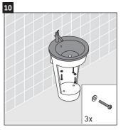
Using three screws and three washernets secure the washbasin to the vanity.
