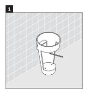
Mark the holes to be drilled for the anchors.
