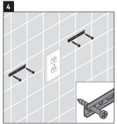
Screw the bracket(s) to the wall at the specified locations. For wood stud walls, bolts should be screwed into wood backing.
