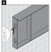
Plug the unit into outlet and lift the unit up and onto the mounting brackets.
