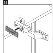
Re-attach plate with Duravit logo. Installation is complete. Furniture complies with applicable requirements of the referenced standard(s): Safety Household and Commercial Furnishings (UL 962, 3rd ed. Issued: 07/07/08, Revised: 08/05/13) Portable Luminaires CSA C22.2 No. 12 - 1982 (R2004)
