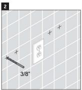
Using a 3/8" drill bit, drill the anchor holes that have been marked.
