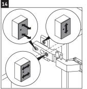
The top screw will adjsut up and down. Back screw will adjust closer and further from the mirror cabinet and front screw will adjust left and right.
