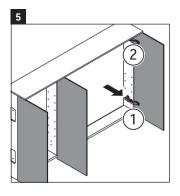
Prior to mounting, remove the mirror front(s) of the cabinet by unlatching each hinge. Also remove side panels.
