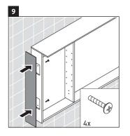
Attach side front with four supplied screws.
