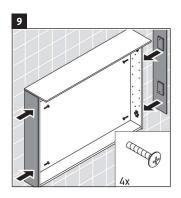
Attach side fronts with four supplied screws.
