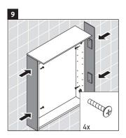
Attach side fronts with four supplied screws.
