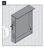
Plug the unit into outlet and lift the unit up and onto the mounting brackets.
