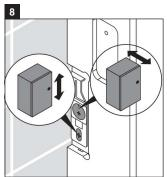
Check the screws which allow adjustment of the unit. The top screw will adjust front to back and the bottom screw will adjust up and down.
