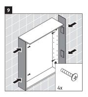
Attach side fronts with four supplied screws.
