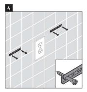
Screw the bracket(s) to the wall at the specified locations. For the wood stud walls, bolts should be screwed into wood backing.
