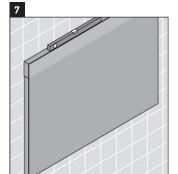
Check the mirror is leveled and securely attached to the wall.
