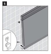
Plug the mirror into the outlet and line up the mounting hooks with the inserts on the back of the mirror. Push mirror onto wall until hooks are inserted securely.
