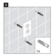
The plastic anchors provided are for concrete wall applications.
