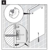
Lay the bottom of the mirror against the wall and tighten the set screw to secure the mirror in place.
