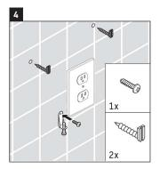
Thread the two mounting screws into top two anchors, leaving hooks facing up.
