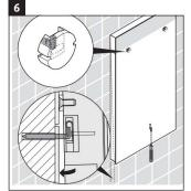
Lay the bottom of the mirror against the wall and tighten the set screw to secure the mirror in place.
