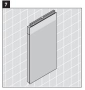
Check the mirror is leveled and securely attached to the wall.
