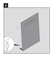
Plug the mirror into the outlet and line up the mounting hooks with the inserts on the back of mirror. Push mirror onto wall until hooks are inserted securely.
