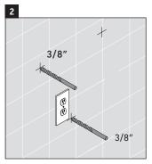
Using a 3/8" drill bit, drill the anchor holes that have been marked.
