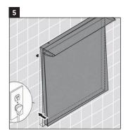
Plug the mirror into the outlet and line up the mounting hooks with the inserts on the back of the mirror. Push mirror onto wall until hooks are inserted securely.
