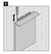
Use the adjustment tool to move mirror up and down for the leveling.
