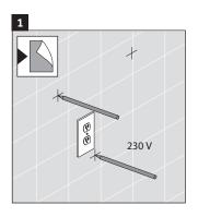
A 110 V GFCI outlet is required. Mark the holes to be drilled for the anchors.
