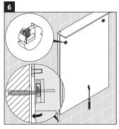
Lay the bottom of the mirror against the wall and tighten the set screw to secure the mirror in place.
