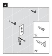
Thread the two mounting screws into the top two anchors, leaving the hooks facing up.
