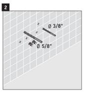
Using a 3/8" and 5/8" drill bit, drill the anchor holes that have been marked.
