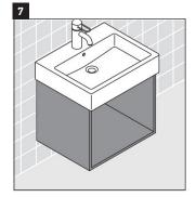
Slide the vanity under the washbasin. Tighten mounting bolts with a wrench until the washbasin is stable.
