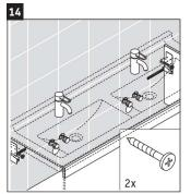
For wood stud walls, bolts should be screwed into wood backing.
