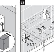
Using the appropriate bit for the wall material, drill pilot holes.
