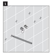
Reference the washbasin specification to establish the position of mounting bolts, mark the holes to be drilled for the anchors.
