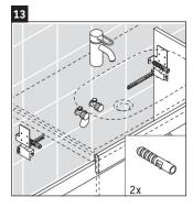
The plastic anchors provided are for concrete wall applications.
