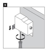
Using a crewdriver adjust the vanity mounting hinge system counter-clockwise.
