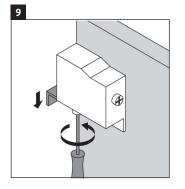
Using a crewdriver adjust the vanity mounting hinge system counter-clockwise.
