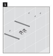
Reference the washbasin specification (page 1) to establish the height and spacing of the mounting bolts.
