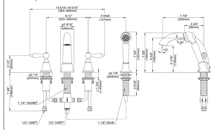
\* Danze Soft Touch Personal Shower™ is designed to operate only when the button is pressed; water will flow to the spout whenever pressure is released from the button.
