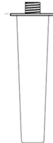
RECESS CONNECTION 1/2" NPT (MALE THREAD)
