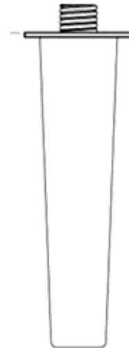
RECESS CONNECTION 1/2" NPT (MALE THREAD)
