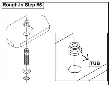
Apply teflon tape or pipe joint compound to the short end of the 3/4" spout nipple. Thread short end of the nipple into the quick connect deck spout adapter. Install the quick connect adapter through the 1-1/4" hole in the deck making sure that the deck spout adaptor sits flat on the finished deck
