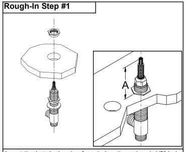
Insert the hot deck valve from below through a 1 1/2" hole and install the top-fastening nut. Set the deck valve to proper rough-in height by adjusting the top mounting nut and secure the valve by tightening the bottom valve nut. The rough in measurement is found by using measurement 'A' on the Rough In Specification sheet on the back of this pamphlet. The trim product number must be known. The stem and nipple may be trimmed to arrive at the correct rough-in measurement.
