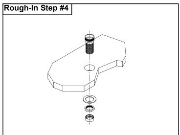
Install the nipple for the hand shower hose guide through a 1-1/4" hole in the deck. This should be installed as close as practical to the deck diverter and so that the hand shower (6" center to center) will spray into the tub when in the bracket.
