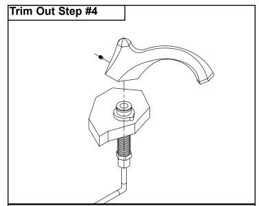
Set the deck spout onto the quick connect spout adapter and tighten the set screw at the base of the spout with the supplied allen wrench.
