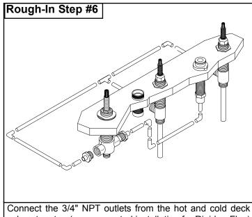
Connect the 3/4" NPT outlets from the hot and cold deck valves to a tee (see suggested installation for Rigid or Flex) and run combined supply to the "INLET" port on the deck diverter valve. Connect the port marked "OUTLET" on the deck diverter to the deck tub spout nipple.
