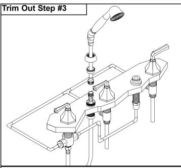
Insert the black plastic insert and loosely attach trim ring to the hose guide for the hand shower. Attach the finished hand shower hose end with the "O" ring to the hand shower. Attach the remaining end to the male end of the stainless steel hose and route both hoses through the hose guide. Place the hand shower so that the head will spray into the tub and hand tighten the trim ring on the hose guide.
