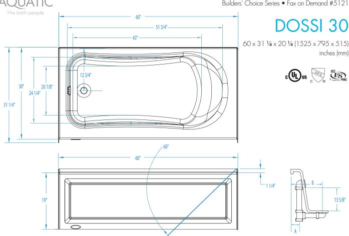
FEATURES Ibs (kg) Dimensional Tolerance ± 38". Dimensions needed for site preparation should be measured from the unit. Aquatic assumes no responsibility for preparatory work.
