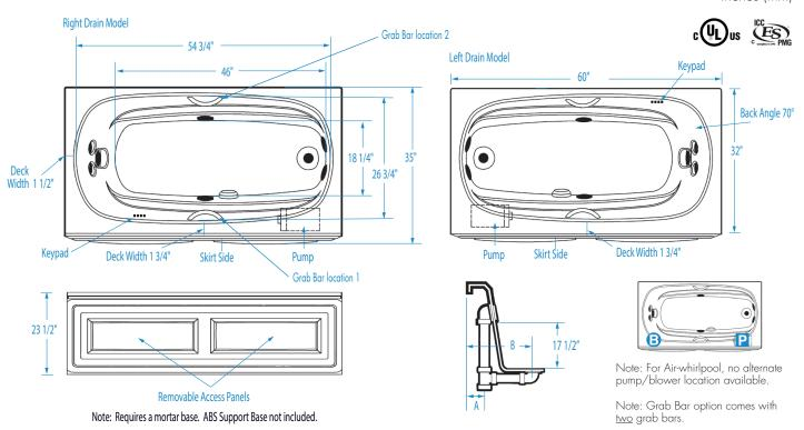
FEATURES lbs (kg) Dimensional Tolerance ± 3/8". Dimensions needed for site preparation should be measured from the unit. Aquatic assumes no responsibility for preparatory work.
