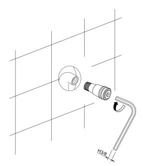
**1**. Slide the adaptor over the stub-out pipe and screw onto the threaded end. Tighten it with 3/8" Hex Wrench (not included).
