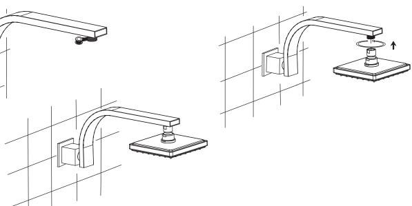
Wrap pipe sealant tape around threads and install showerhead. Tighten securely.
