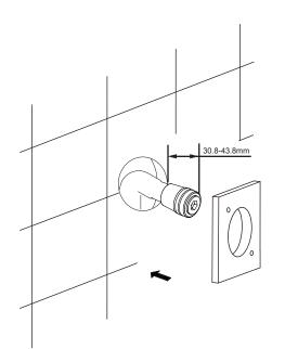
2. Slide wall escutcheon over the stub-out pipe to cover the wall hole.
