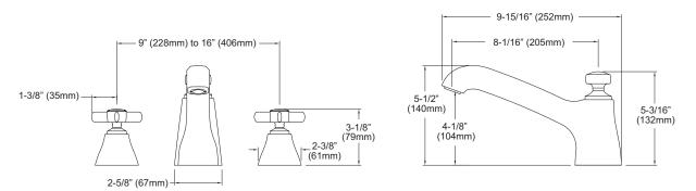
IMPORTANT NOTE: This valve/trim can only be installed in a built-up deck. It cannot be installed on pre-finished deck or on tub rim.
