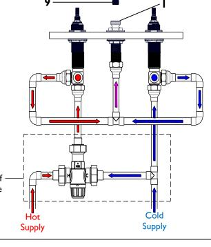
Typical installation of ASSE 1070 tempering valve (follow tempering valve instructions)
