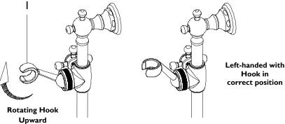
• After orientation is determined, the handshower HOOK (I) must be rotated in up position as shown above.
