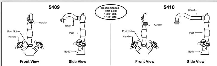
Fig. 1 Meets A112.18.1 - 2.2 gpm/8.31 L/min. \*\*\*NOTE: SHUT OFF WATER SUPPLY BEFORE BEGINNING INSTALLATION\*\*\* Fig. 2
