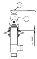
Assemble the handle set (G) screwing the cap (F), placing it in the correct position.
