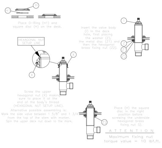
Tighten the trim cap (F) and square disc (H) snugly so cap (F) is in proper alignment with square disc (H) on the deck. Tighten hexagonal brass fixing nut (Z2) under the deck the secure the valve body (I) into the final assembled position. This final adjustment may take a few attempts for the installer to achieve the proper dignment and height of all components depending on the thickness of the deck.
