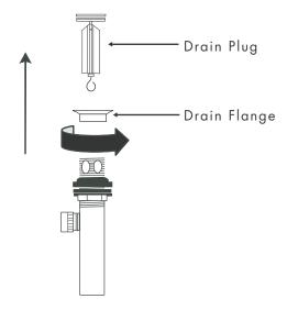
Apply a ring of silicone caulking to underside of Drain Flange. Do not use plumber's putty, which can damage finish.
