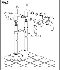
Installation requirements: 2 x1/2" NPT male stub outs at 5 29/32" centers
