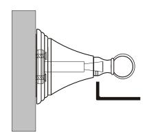
5- Check both roller posts to make sure they are firmly secured. If not, tighten the set screws with the Allen key.
