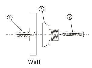
4- Put the bracket ball end in to the hole. It will be seated on the concave disk.
