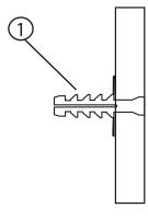
2- Put in the screw though the bracket base into the plastic toggle already mounted in the wall.
