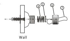
5- Thread on bracket nut on the bracket base.
