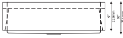
KHF200-33 32 7/8" x 20 3/4" x 10" Min Cabinet Size: 36" Matching Grid: KBG-200-33 Drain Model #: BST-1
