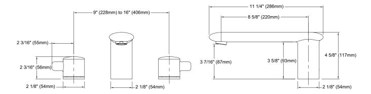
IMPORTANT NOTE: This valve/trim can only be installed in a built-up deck. It cannot be installed on pre-finished deck or on tub rim.
