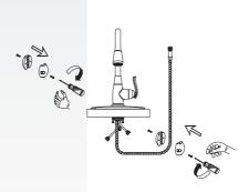
Attach metal weight to hose to prevent hose from twisting and returns hose to proper position.
