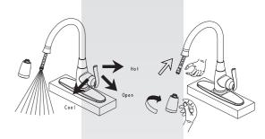
After installing faucet, remove pull-down spray and turn on water to remove any left over debris. Re-assemble spout.
