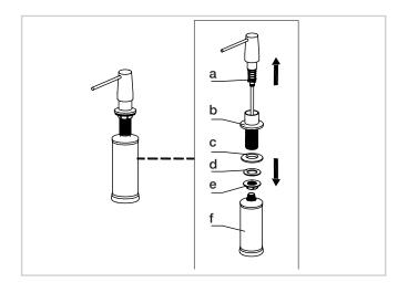
Install dispenser base (b) with rubber washer A (c) attached into the hole in the countertop. Re-install rubber washer B (d) and mounting nut (e) on the dispenser base (b) from underneath the countertop. Tighten mounting nut (e) with adjustable wrench until snug
