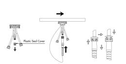
Remove the plastic seal cover from the outlet port prior to pushing the hose adapter onto the same port, you will hear a "click" sound once they are
