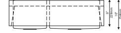
KHF204-33 32 7/8" x 20 3/4" x 10" Min Cabinet Size: 36" Matching Grid: KBG-204-33-1 and KBG-204-33-2 Drain Model #: BST-1 & ST-1
