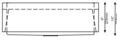
KHF200-30 29 3/4" x 20 3/4" x 10" Min Cabinet Size: 33" Matching Grid: KBG-200-30 Drain Model #: BST-1
